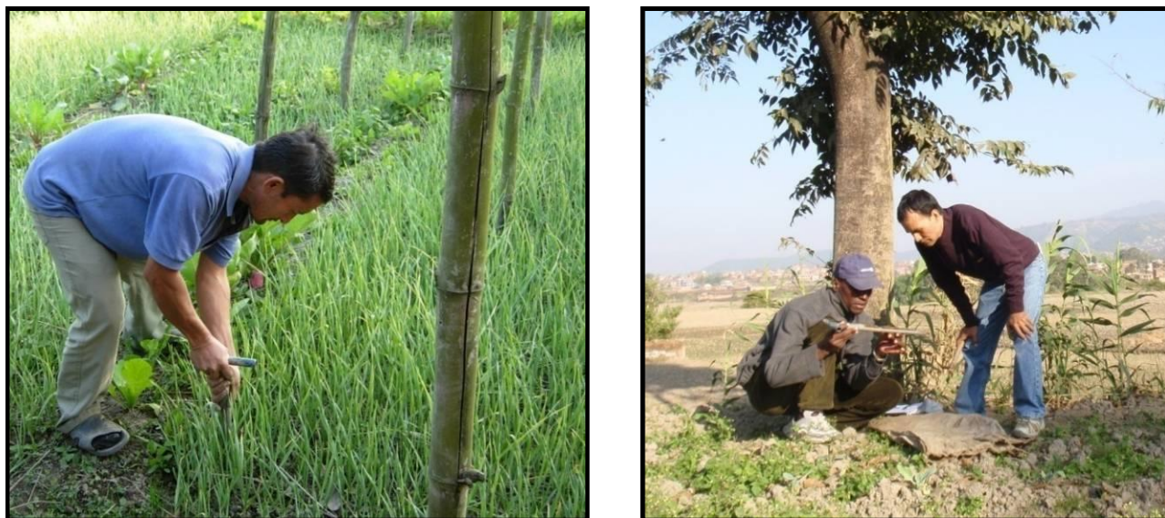
Figure 3.1 Soil sampling using the hand probe from fertilized (L) and unfertilized areas (R)
