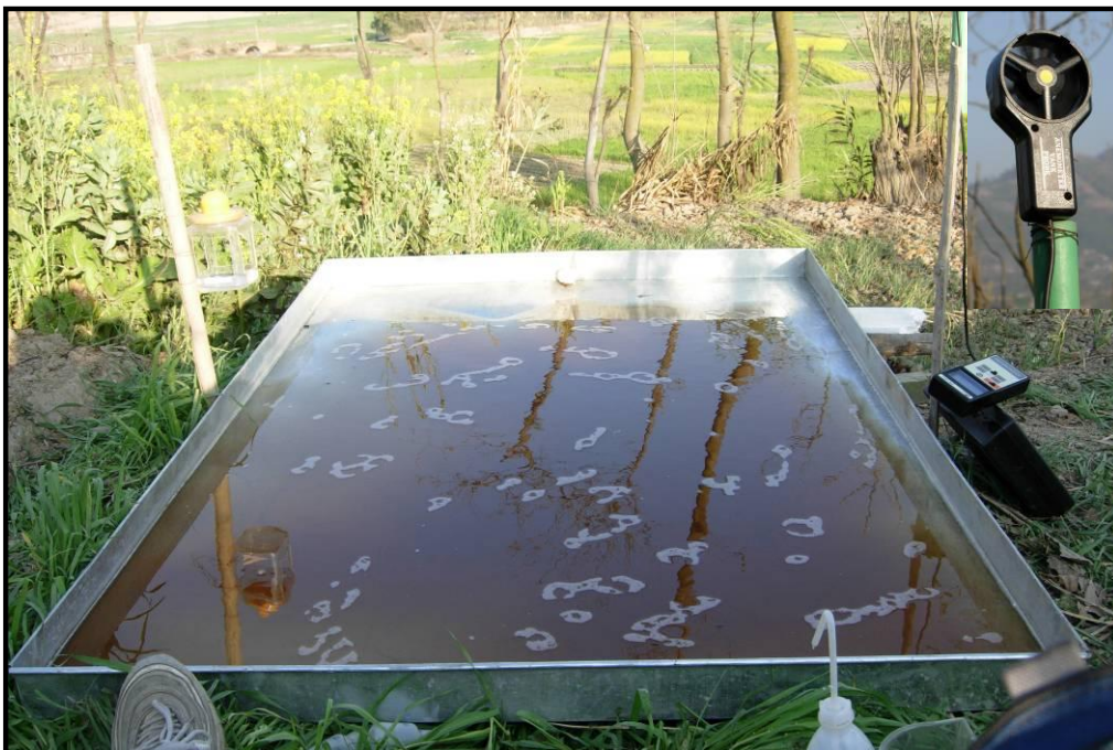
Figure 3.4: Ammonia basin at reference point with trap and anemometer on sideline.
